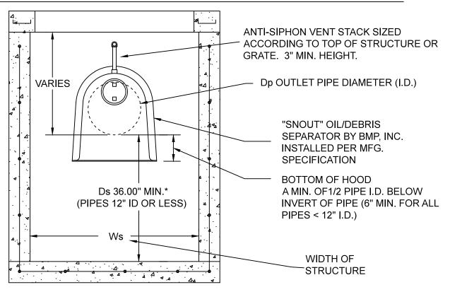
RULE # 1- AT AN ABSOLUTE MINIMUM, STRUCTURE INTERNAL DIMENSIONS MUST BE AT LEAST LARGE ENOUGH TO ACCOMODATE EXTERNAL DIMENSIONS OF THE SNOUT, AND ALLOW FOR A PERSON TO INSTALL IT. REFER TO BMP, INC. CAD DETAILS FOR PART DIMENSIONS. BMP RECOMMENDS STRUCTURE WALL TO BE AT LEAST 12" WIDER THAN MAXIMUM SNOUT WIDTH. FOR TRASHSCREEN, STRUCTURE MUST BE AT LEAST 6" WIDER THAN TRASHSCREEN WIDTH.
