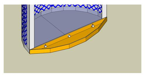
Bolt the Adapter Tray to the back flange of the Stainless TrashScreen<sup>™</sup>, with the enclosed 3/8" bolts and nuts
