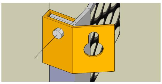
Attach the 2 hanger clips to the existing keyhole slots at the top of the Stainless TrashScreen<sup>™</sup> frame with the enclosed 3/8" bolts and nuts. (Pay attention to left and right handed keyholes)
