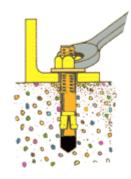
3. Tighten nut until wrench resistance is felt (approximately 3 to 4 turns of the nut after snugged up) anchorage is now complete.
