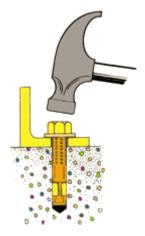
2. Place nut on the end of the wedge anchor (to protect the threads of the wedge anchor during installation)
